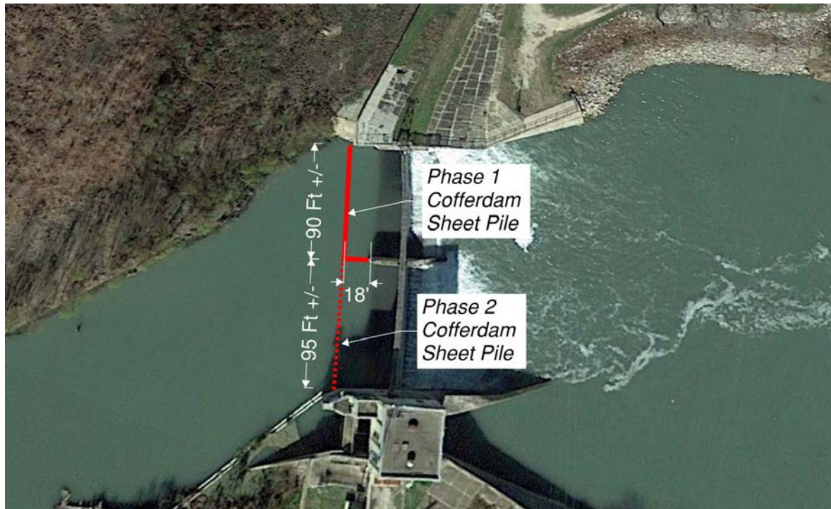
Figure 6-4 Construction Cofferdam Option 3 – Sheet Pile Plan
